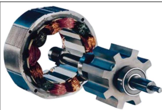
Figure 43: A 3 phase, 2 pole pair, 12-8 SRM (25)
